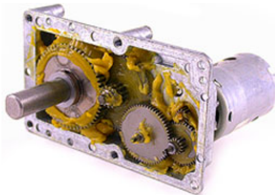
Figure 40: Inside Mechanism of Motor and Gear Set (Permission Pending)
